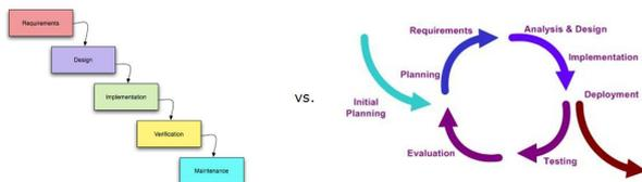
Figure 2: “Waterfall” vs. “Concurrent” engineering process
