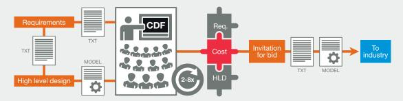
▲ The concurrent design process is quite different from the waterfall process. Requirements, design and cost estimates are all 'locked down' at the same time. This allows the requirements to be adapted so that they meet the user requirements and also results in an optimal design.
